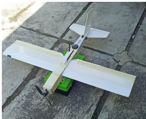
Fig. 6. Fixed wing UAV model that used to capture data.
