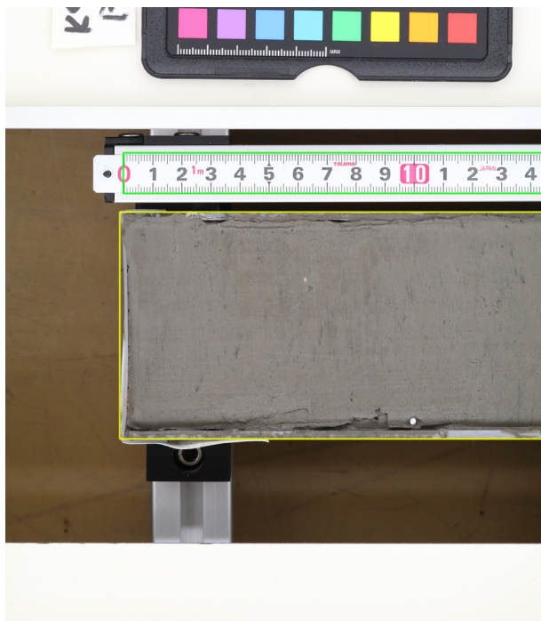
Fig. 1. Core scanner output with actual core (yellow rectangle) and scale (green rectangle).
