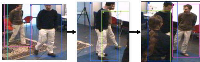
Fig. 15: FastMOT continuing to track despite occlusion
