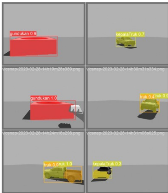
Fig. 6: The object detection results depicting detection of vehicle (labelled truk and kepalaTruk ) and the target object (labelled gundukan ).
