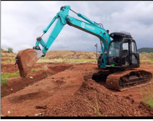
Fig. 1: ASTA Autonomous Excavator by ABAROBOTICS used in this research.
